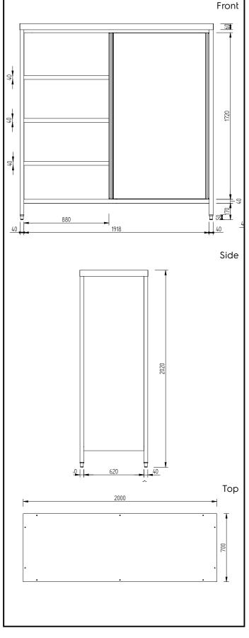
PLUS - Static Preparation 2000 mm Storage Cabinet with sliding doors
